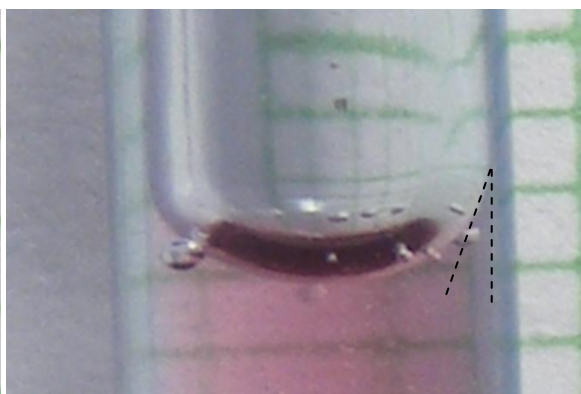
Figure 4: Meniscus, SAE-30 in 3 mm PVC tube; 1) bottom of column 2) top of column. Note leakage out of bottom left of column
