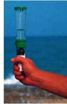
Ventimeter: for airflow strengths from light breeze to gale force.
