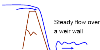
Steady flow: flow is established with all forces in balance on average
