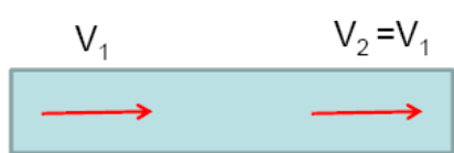
Uniform flow: no change in velocity from point to point
