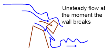
Unsteady flow: accelerations must be accounted for to balance forces
