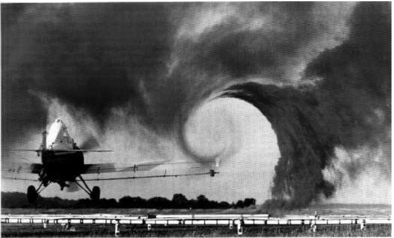
Vortex motion in a cropduster's wake (image courtesy DANTEC measurement Technology Inc.)
