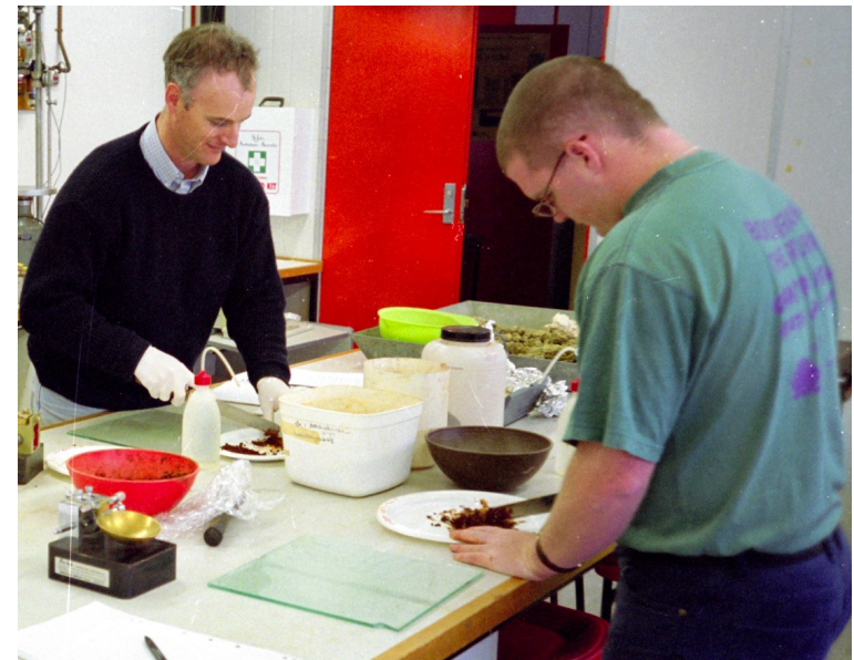
students doing plastic limit tests (RGG)
