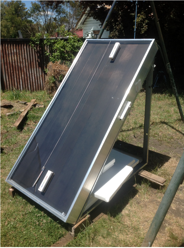
Plate 1: SolrHeat space heater with thermal instrumentation.
